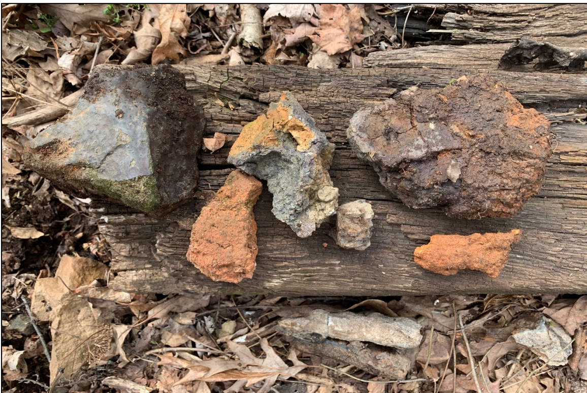
Photo 12. Detail of debris scatter (fire brick/clay slag) found at the base of the furnace.
