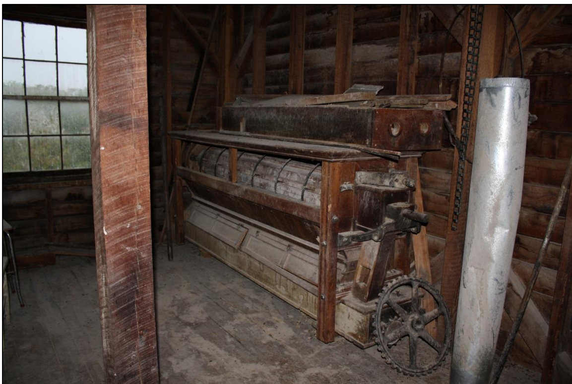
WV_HampshireCounty_French's Mill_0026 French's Mill, Interior, Third Level, Richmond City Mill Works, Rolling Screen, Facing West
