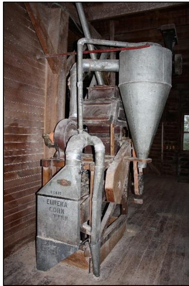
WV_HampshireCounty_French's Mill_0021 French's Mill, Interior, Second Floor Mill Room, Corn Cutter, Facing North
