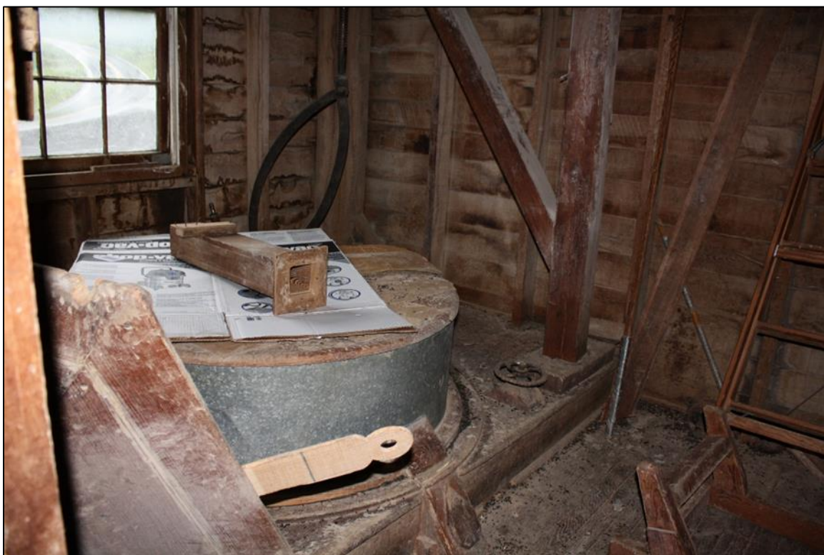
WV_HampshireCounty_French's Mill_0011 French's Mill, Interior, First Floor, Burr Stones, Facing North
