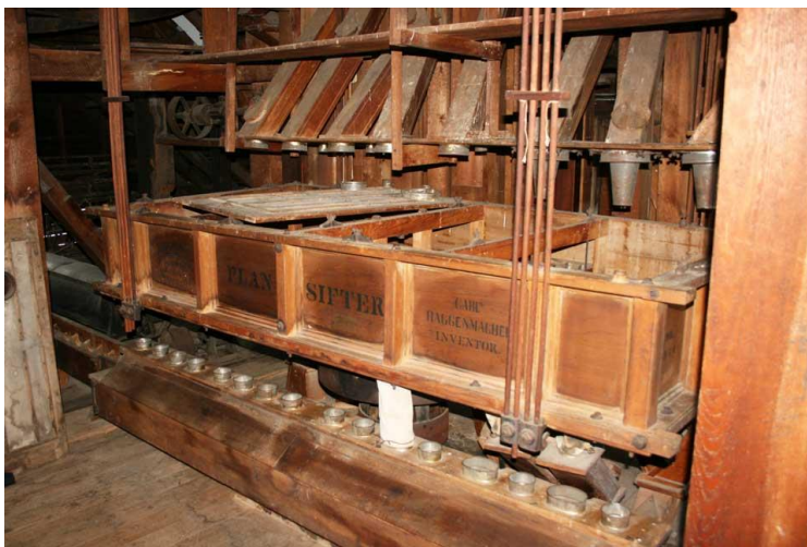
Figure 6. Bernard & Leas plansifter (Carl Hagenmacher, Inventor) in current use (2016) at Thorp Mill, Thorp, Washington. "Thorp Mill," accessed July 17, 2016, http://www.thorp.org/grist-mill-diagram/
